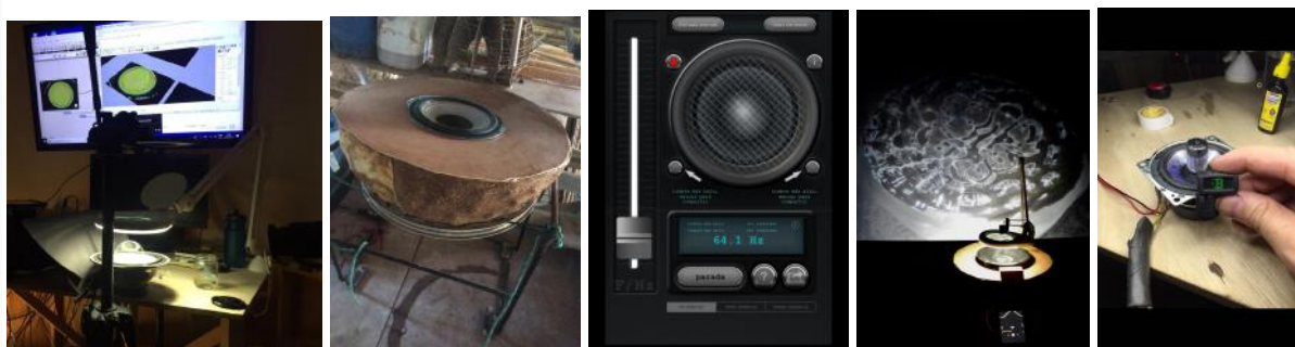
Figure 13,14,15 : Cymatic record session, Tomorrow's Activities Laboratory (Brazil). Set of Cymatic Projection. Speaker made by bamboo internal structure , covered by mud and natural resin (Source: Author).
